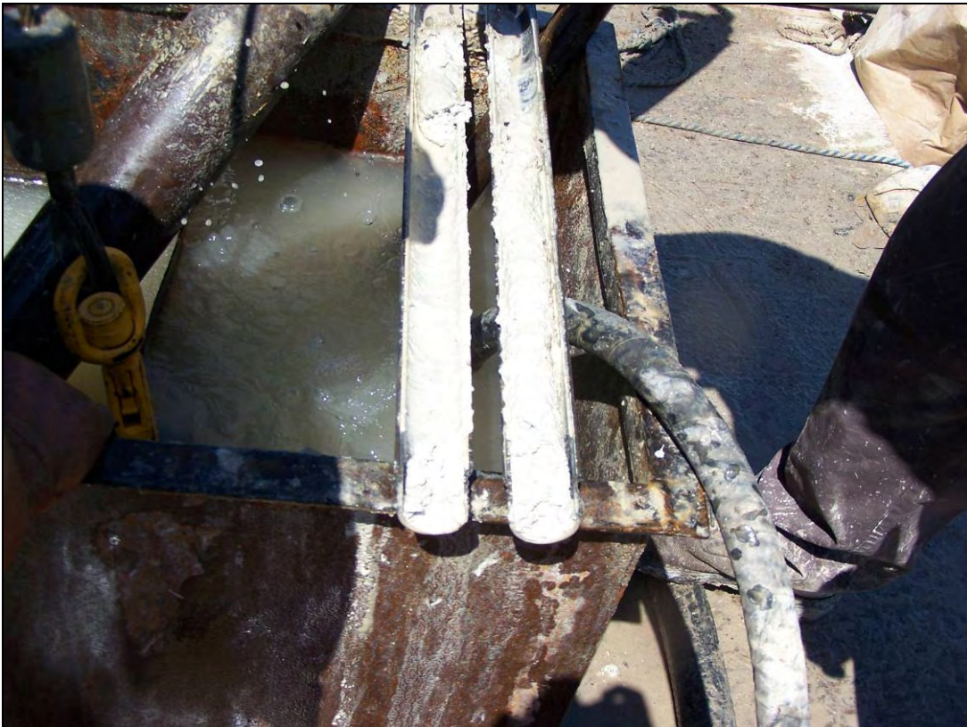
Split spoon recovery from rock boring depth of 6ft to 8ft
