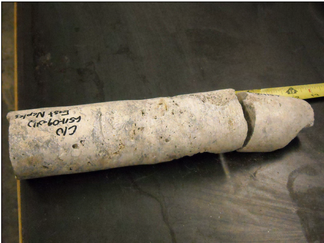
Rock core recovery dried in lab
