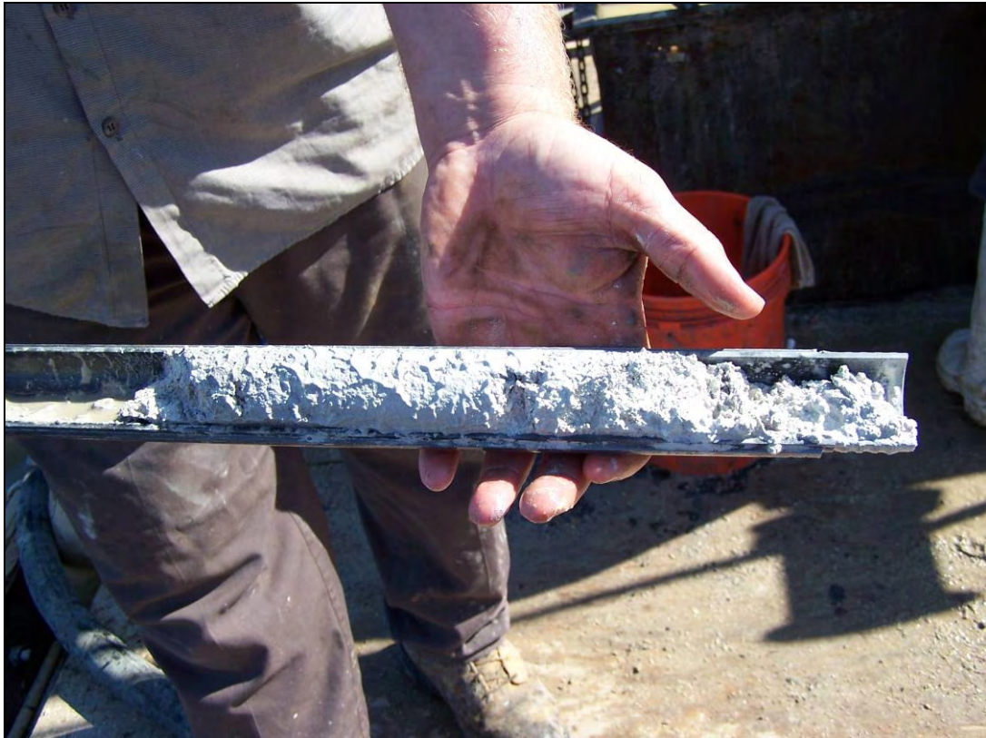
Split spoon recovery from rock boring depth of 2ft to 4ft
