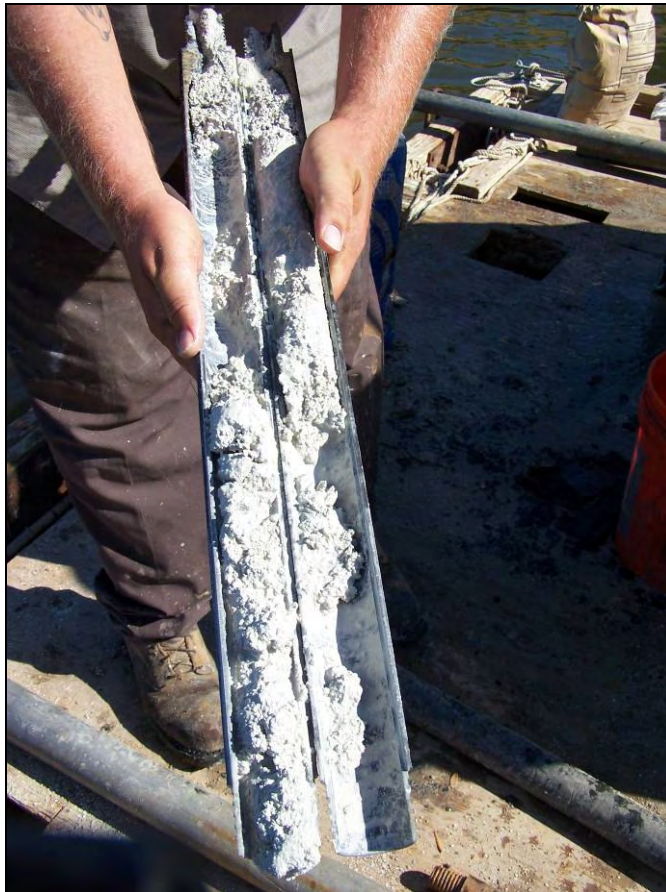
Split spoon recovery from rock boring depth of 6ft to 8ft
