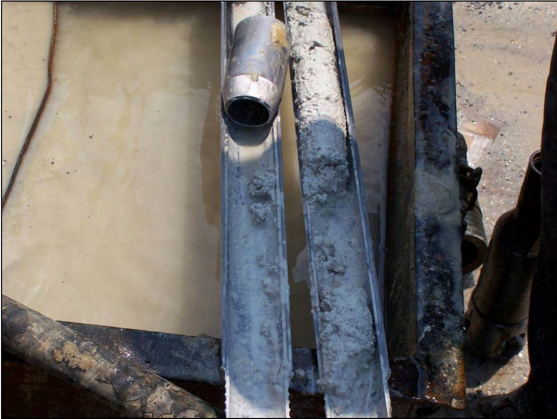
Split spoon recovery from rock boring depth of 4ft to 6ft
