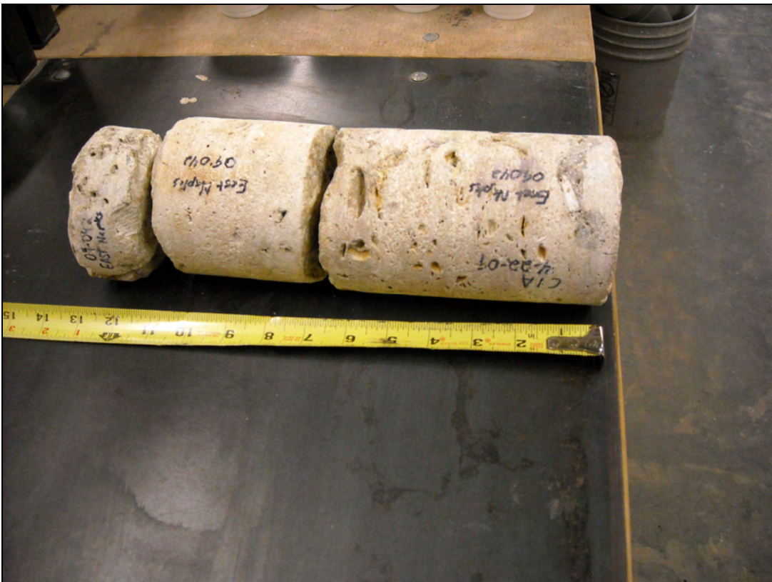
Rock core recovery dried in lab
