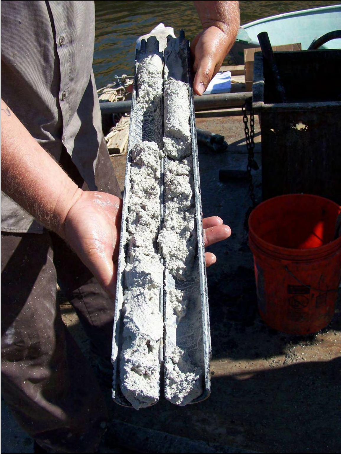
Split spoon recovery from rock boring depth of 0ft to 2ft
