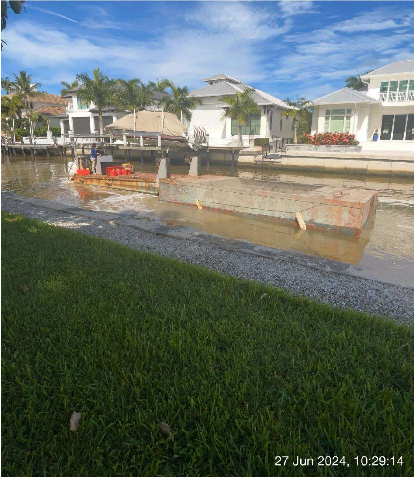
Push boat taking hopper to staging area.
